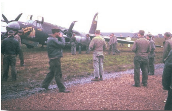
Battle damaged B-26 following an emergency landing. Flak damage caused failure of left main landing gear.
